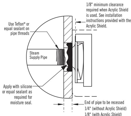
**CAUTION** Consult with supplier of acrylic, fiberglass and other non-heat resistant enclosures for recommended steamhead location. Use Acrylic Shield PN 103938 / 103938SQ. See instructions provided with steam shield. (An acrylic shield is not available for the iSteam steamhead.)
